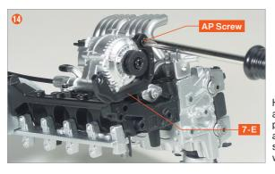
Step complet Hold the assembled alternator and 7-E in place to keep them aligned, match the screw holes, and secure with an AP screw.
