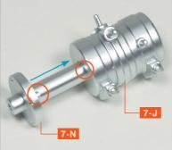
Insert A/C Compressor (3) 7-N into A/C Compressor (1) 7-J, aligning the projection on 7-N with the notch on 7-J, then press them together firmly.
