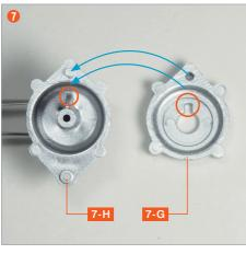
Turn **7-H** over, align the circular recess on **Alternator (2) 7-G** with the screw hole projection on **7-H**, and insert the projection of **7-H** into the hole of **7-G** to secure it.
